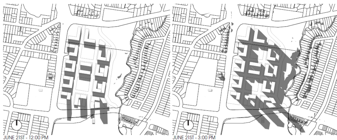
Figure 21 - Overshadowing diagram – 12pm winter solstice (left) and at 3pm winter solstice (right)
